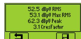
At the end of the acquisition time, a screen detailing RMS, Max RMS, Peak and Crest factor values, is displayed.:
