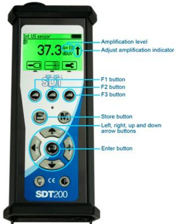
If the acquisition time is set to 0 second, the RMS, Max RMS, Peak and Crest Factor are refreshed every 250 milliseconds. This mode enables the operator to take data on the fly.
