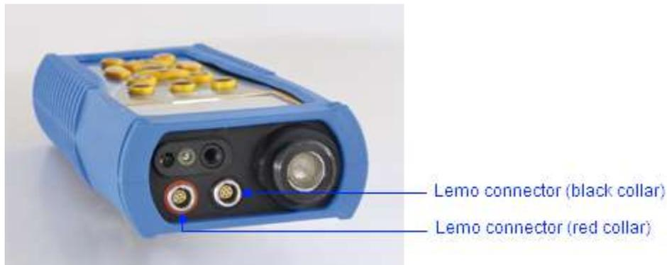
The connections for external sensors are LEMO connectors. They are a commonly used industrial connector, considered for their reliability and their robustness. They have a sprung-loaded knurled barrel and mechanical polarization to go only in one way round
