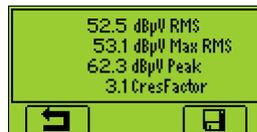
Press the **F3 button** or the **Store button** to save the data (or the **F1 button** to come back to the measurement screen without saving the data)
