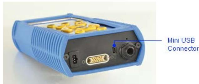
*Back plate of the SDT270 with the Mini USB connector*
