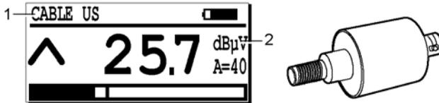
The icon with an ultrasonic external threaded sensor.
