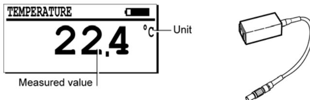
*The Sensor options menu with a thermocouple interface.*
