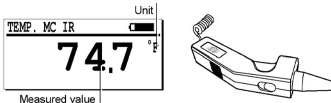
The Sensor options menu with the non-contact infrared temperature sensor.
