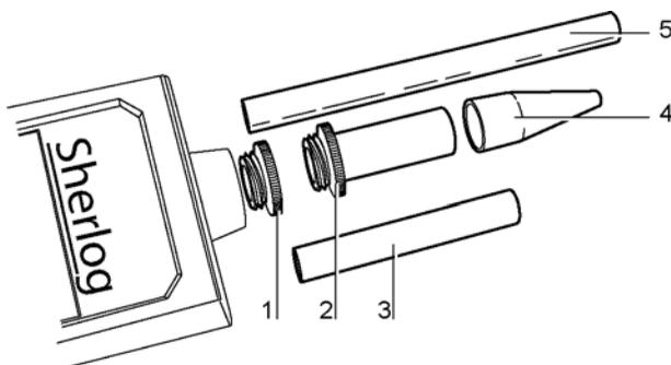
1. Protection cap to be removed before any measurement.
