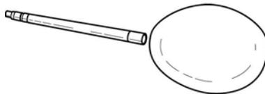
*External view of the sound level meter and its wind bonnet.*
