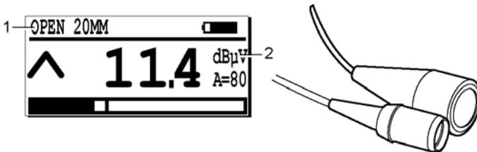
*The specific icon with an ultrasonic external open sensor.*
