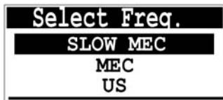
*Example of screen when selecting the measuring frequency band for the contact probe.*
