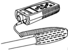
Connect the flexible sensor to the *Sherlog* detector.
