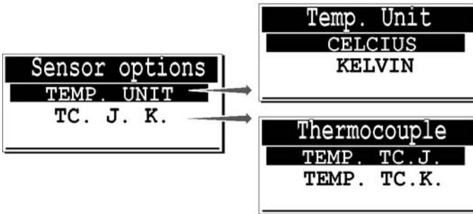
*The Sensor options menu with thermocouple interface.*
