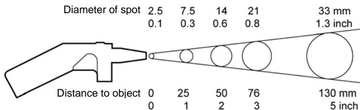
The spot size increases with distance from the probe tip, as shown.
