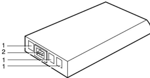
1. Battery contact pads. Do not short circuit.
