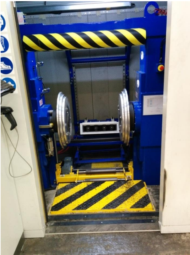
Photo 1 : Front view of the closed chamber. The pneumatically operated door is open. One sees the O4US four sensors mounted inside a metal cone.
