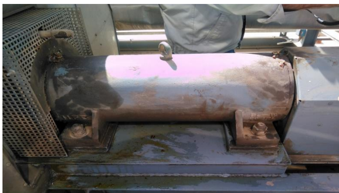
Figure 2 - Two fan bearings with different load. Why do they share the same grease replenishment protocol?
