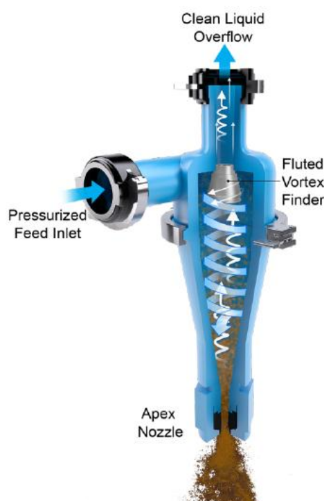
Figure 1: Hydro-Cyclone Components
