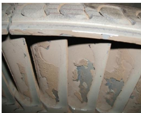
Figure 2 - Scaling on turbine blades
