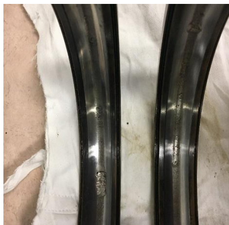
Figure 3 Outer race damage (BPFO)
