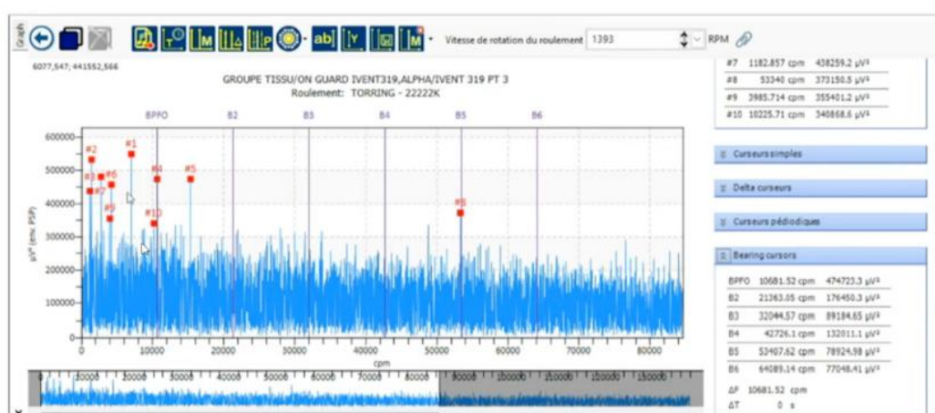
Figure 4: Dynamic Ultrasound Measurement Taken with the LUBExpert Handheld Data Collector & Analyzed in UAS3
