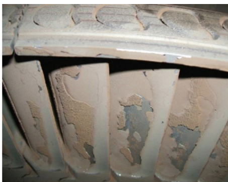
Figure 2 - Scaling on turbine blades
