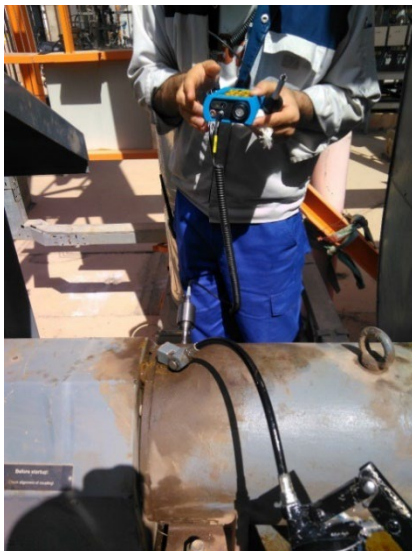
Figure 1 - Collecting ultrasound data with SDT270 while replenishing lubricant.
