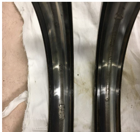
Figure 3 Outer race damage (BPFO)
