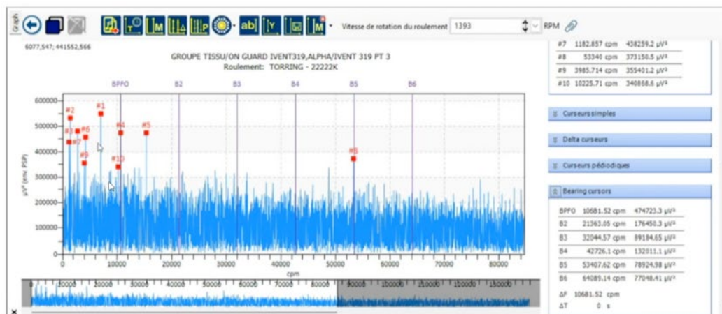
Figure 4: Dynamic Ultrasound Measurement Taken with the LUBExpert Handheld Data Collector & Analyzed in UAS3
