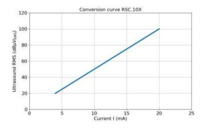
**Note**: Quiet environments below 20[dB<sub>µV RMS</sub>] are not quantifiable by these sensors. Measuring 4 mA indicates that the surrounding environment is below or equal to 20[dB<sub>µV RMS</sub>]. Similarly, noisy environments above 100[dB<sub>µV RMS</sub>] are not quantifiable by these sensors.
