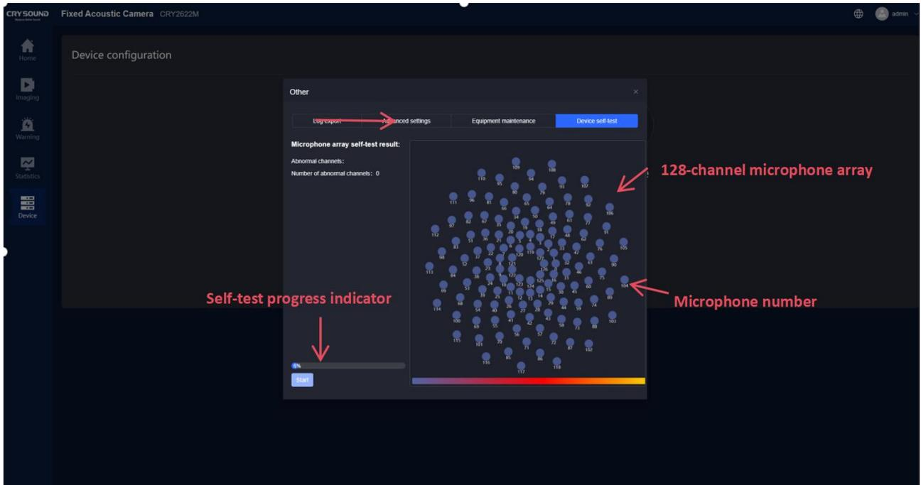
Click the Start Self-Test button to display a self-test process progress bar above the Start Self-Test button. The self-test process takes 90-120S.
