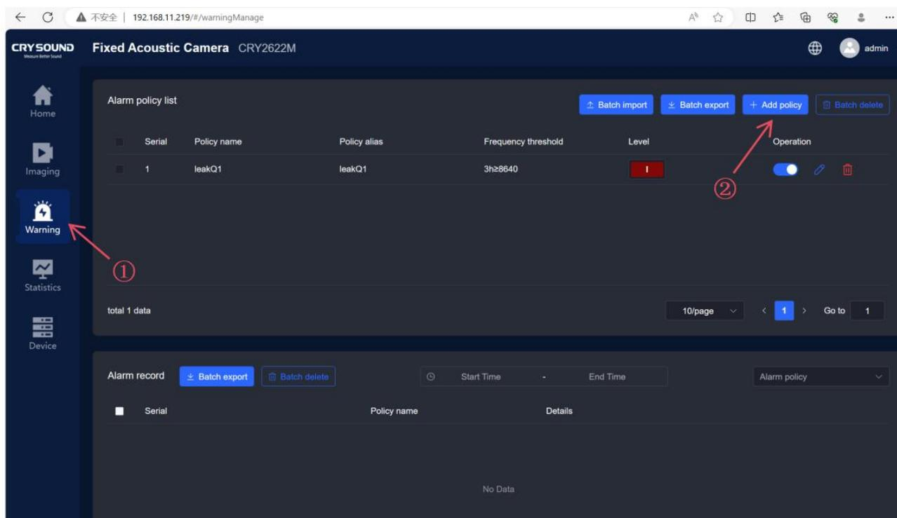
The screenshot shows the web interface for a Fixed Acoustic Camera (CRY2622M). The main content area displays the "Alarm policy list" with a table containing one entry:
