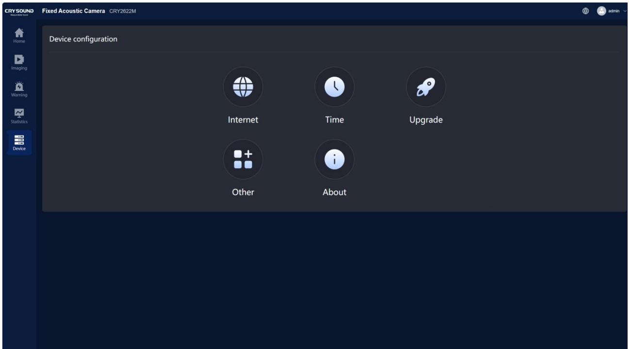
The device configuration is mainly divided into the following five parts: Network, Time, Firmware Upgrade, Other, About.
