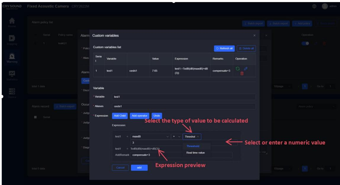
3.3. Preview the expression of the custom variable, where dB(x) means that the unit of the current variable x is dB, and TodB(y) means that the output value of the current variable y is in dB.
