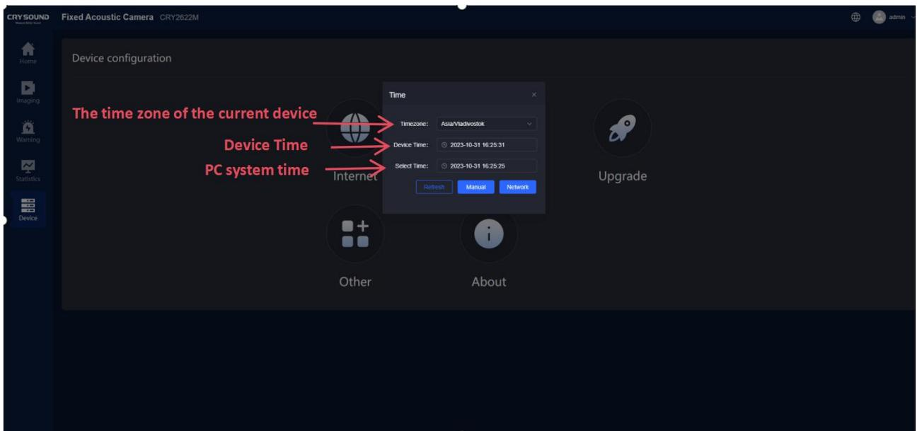
On the time setting interface, the three display boxes are; Current device time zone, current device time, PC system time.
