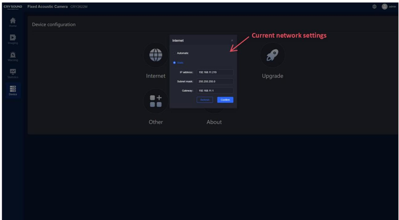
The network can be set to automatically obtain IP address mode (O) or use the following IP address pattern (P). As shown in the figure P static address mode, the current network configuration is displayed by default when the window is opened.
