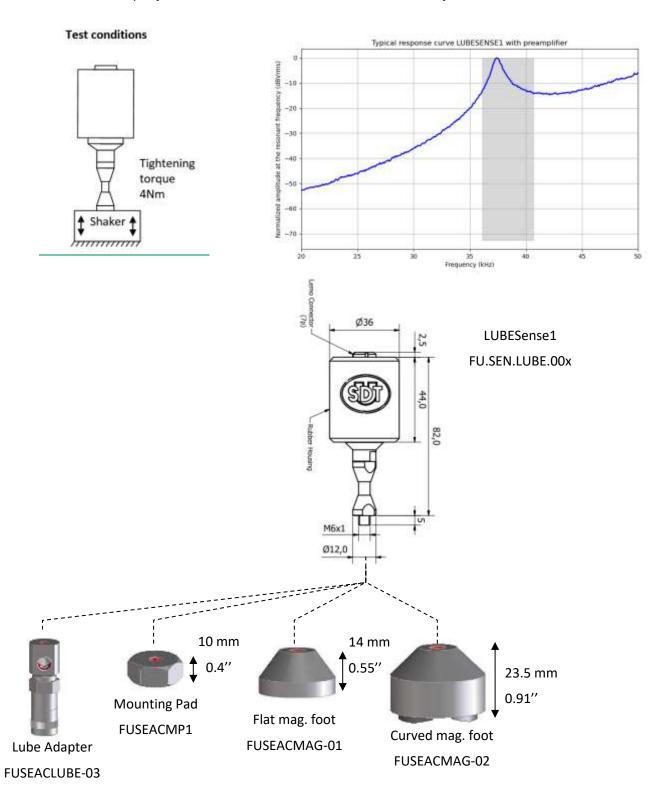
The foot is a part of the resonant structure, please do not disassemble it!
