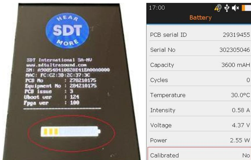
If you've identified a battery calibration fault, a full battery charge is required. Follow these steps to perform a full battery charge:
