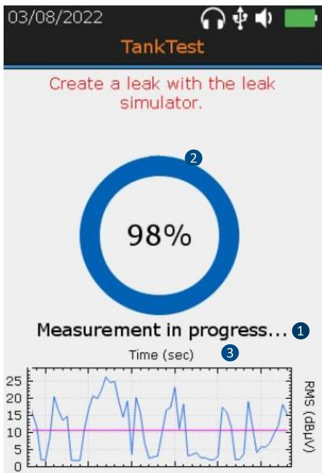
① Acquisition screen (trigger with the **Enter** key)
