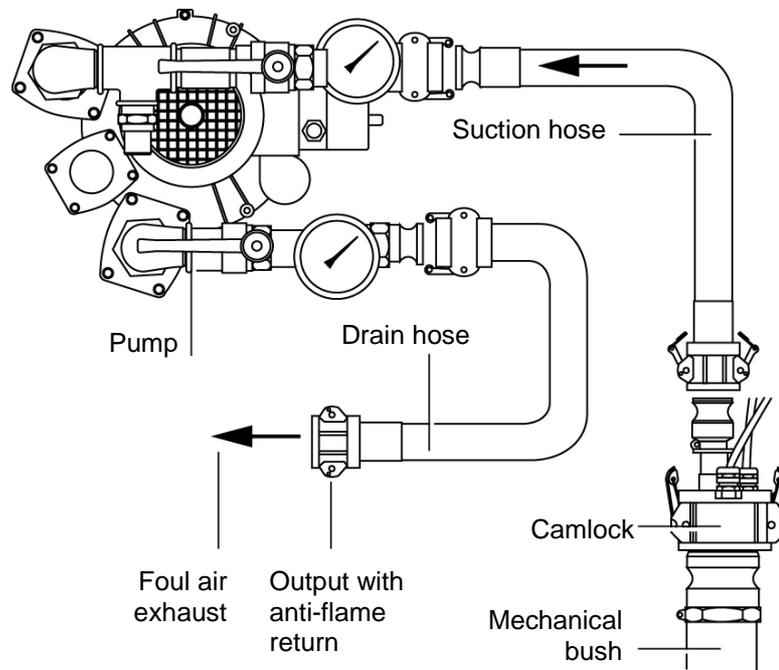
Figure 21 : Connection of piping to the vacuum pump (non-flame-proof version) and to the camlock.
