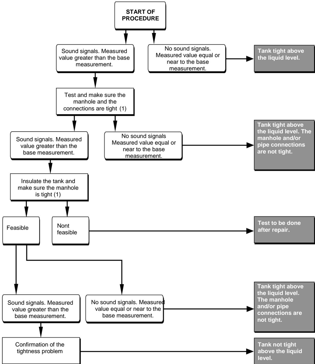
Figure 24 : Test above the liquid level.
