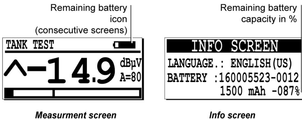
Figure 13 : Example of battery capacity remaining.
