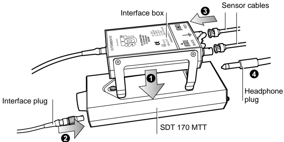
Figure 16 : The interface is positioned under the SDT 170 MTT and connected to the latter and the two ultrasonic sensors.
