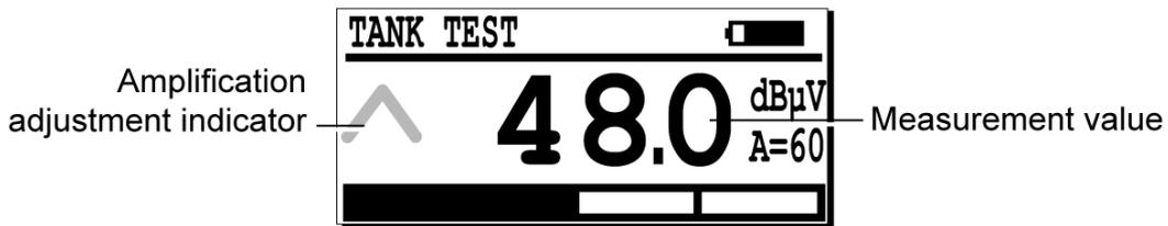
Figure 19 : Arrow signs will disappear when the level of amplification is right and the measurement value reaches at least 40 dB $\mu$ V when pressing the thumb on the sensor. 511
