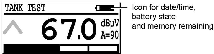
Figure 10: Location of icons for date, time, battery state and memory used.
