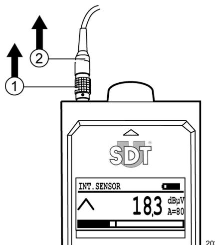
Note: the cable of the flexible rod is also equipped with a 7 pin LEMO plug.
