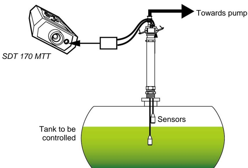
Figure 5 : Principle of ultrasonic tightness controls.
