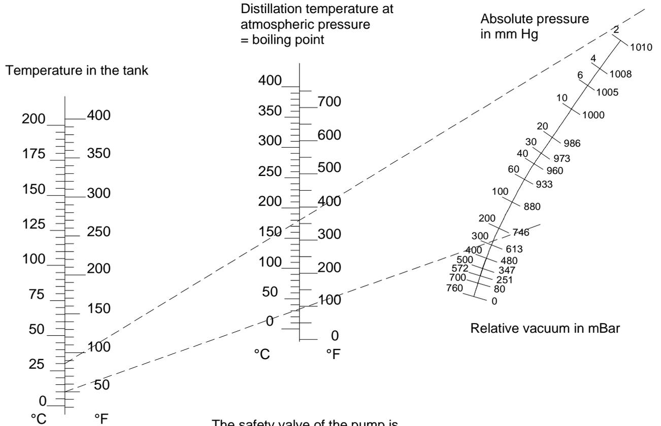
The safety valve of the pump is pre-set at 250 mBar relative to avoid damaging the tank
