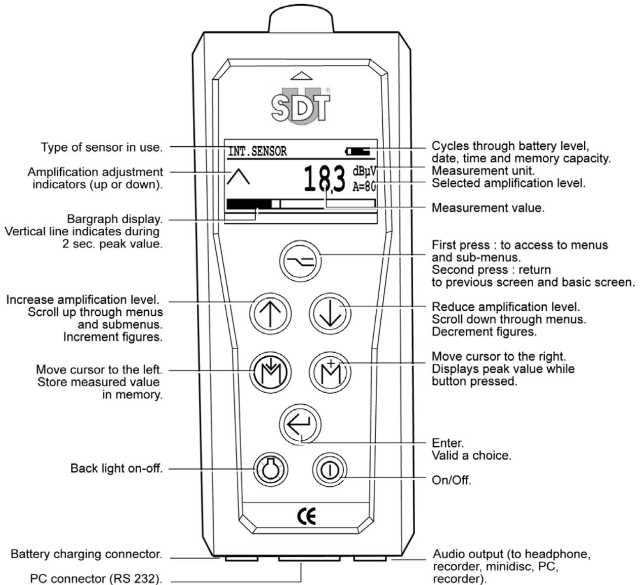
Figure 8 : The function of the main components of the SDT 170 MTT.
