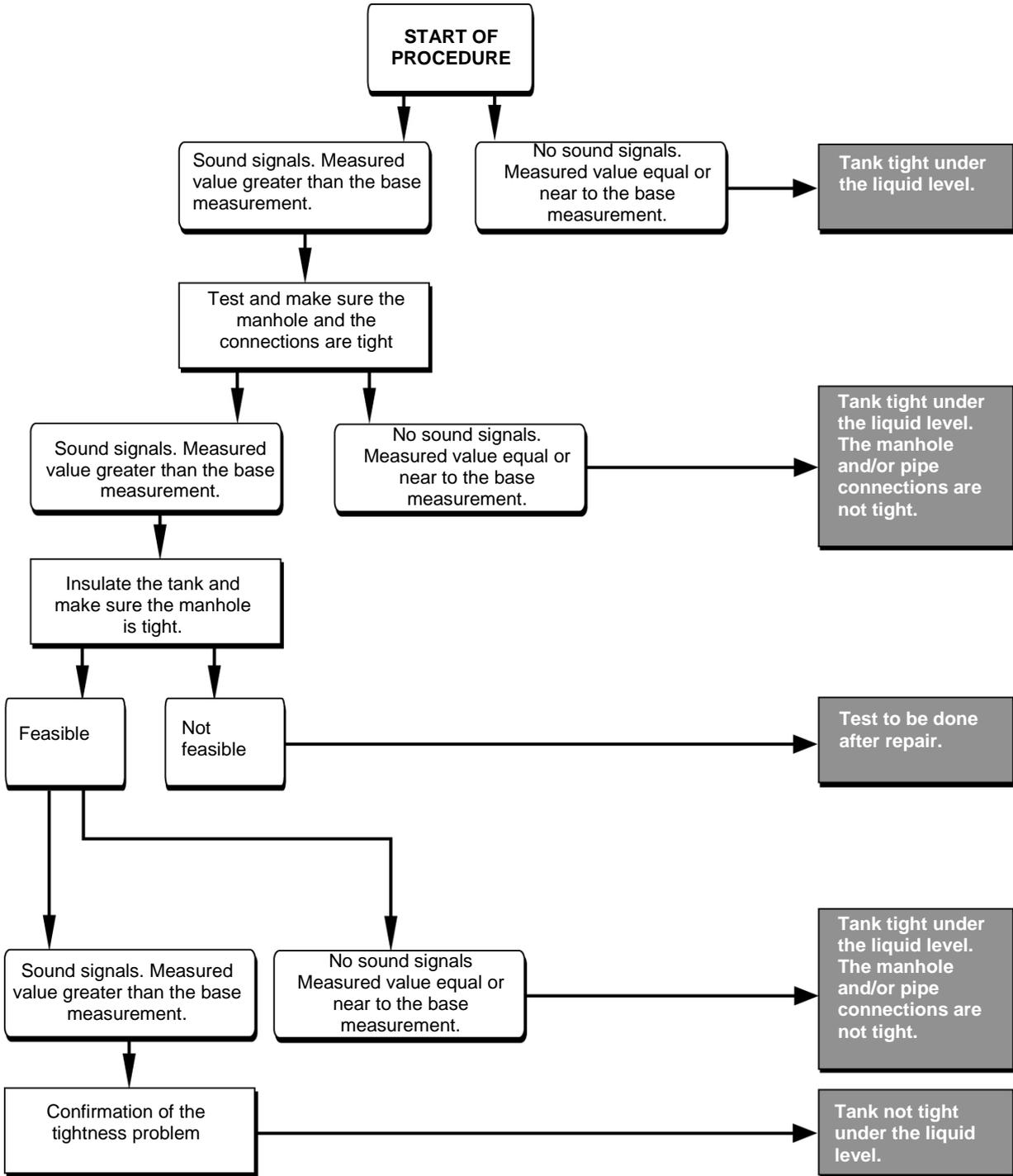
Figure 23 : Test under the liquid level.
