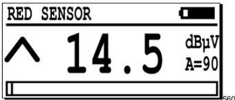
560   | <p>The measuring starts automatically with the submerged sensor (<b>Red sensor</b>). The top left part of the screen indicates alternately &lt;Red sensor&gt; and &lt;Tank test&gt;.</p> <p>The <i>SDT 170 MTT</i> then does one measurement per second. Each measurement is then memorized for the duration of the test laid down in step 5 of § 12.2.</p> |
