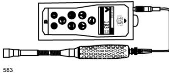
Disconnect the connector of the interface box and connect the flexible sensor.
