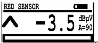
**No noise:** if during this period any characteristic noise is picked in the headphone and a measured value equal or near to the reference value is displayed by pressing the key, this indicates that the tank is tight below the level of the liquid.
