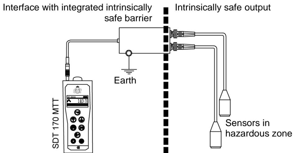
Figure 22 : The interface acts as a galvanic separation between the electrical parts linked to the inside of the tank (sensors) and the measurement device (*SDT 170 MTT*). 507
