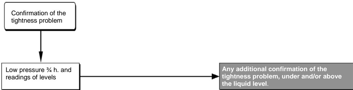
Figure 25 : Depressurize the tank for confirmation of tightness defect(s).
