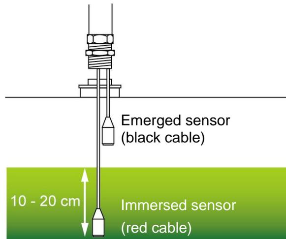
Figure 15 : Position of sensors in and out of the liquid.
