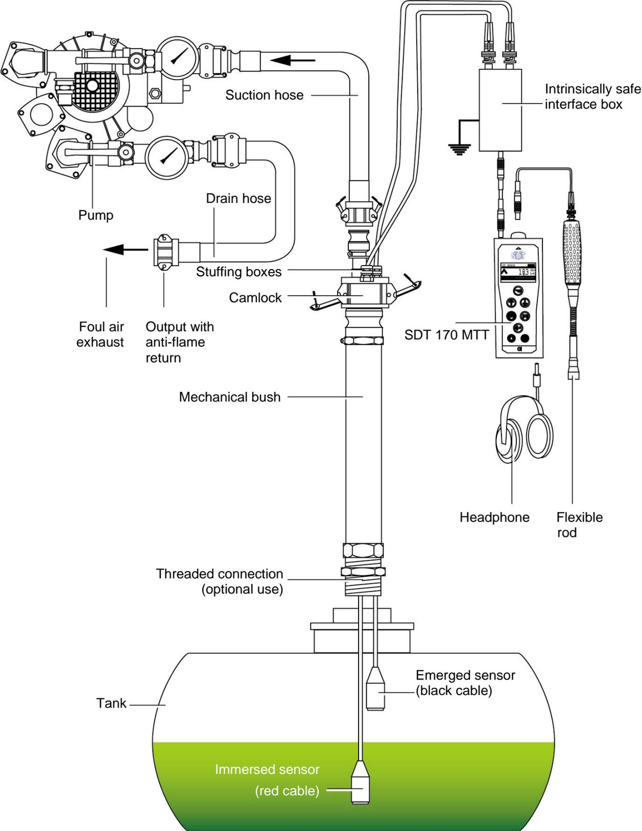
Figure 6: Interconnection of the various parts.
