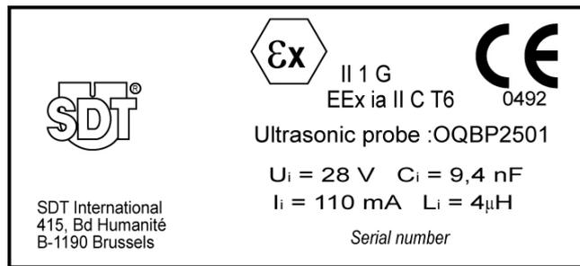
Figure 33: Detail of marking on sensors.
