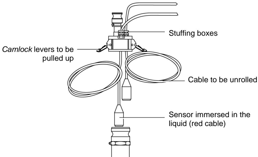
Figure 20 : Introducing sensors and fixing the camlock.
