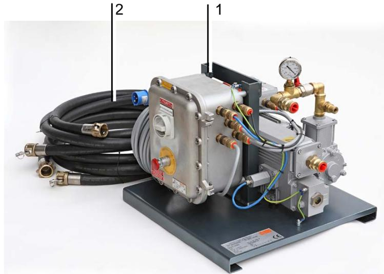
Figure 3 : Optional flameproof equipment: (1) ex-proof vacuum pump, (2) suction and exhaust hoses.
