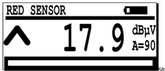
**Presence of noise:** if, during this period, sound signals are heard in the headphone and a value greater than the reference value is shown on the display by pressing the key, this indicates to find the origin of these signals before confirming that the tank is actually perforated below the level of the liquid. Insure that the installation is tight on the surface.
