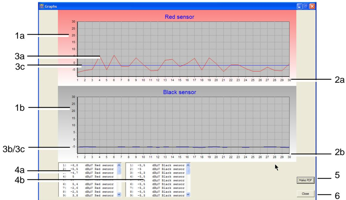
Figure 28: Example of data displayed in graph form.
