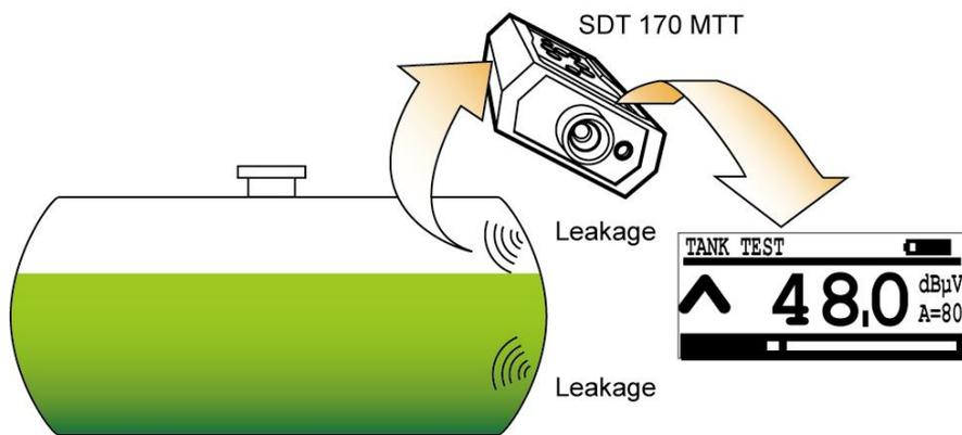
Figure 2 : Any defects in terms of tightness will produce a signal that is detectable by the SDT 170 MTT.
