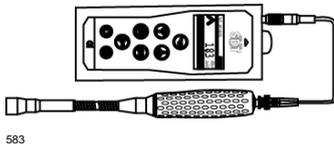
Disconnect the connector of the interface box and connect the flexible sensor.
