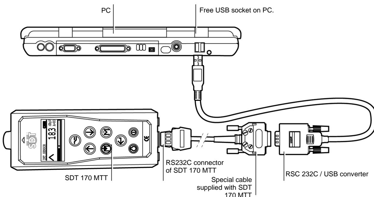
Figure 12: Principle of a *SDT 170 MTT* connection to a USB converter.
